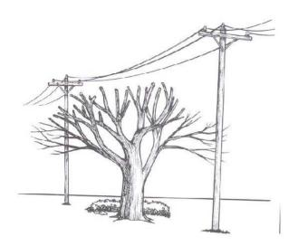
Rounding over, topping, or stubbing branches (left) severely damages trees and is not an approved practice at SYNERGY NORTH. Trees respond to these practices with rapid re-growth of weak branches (right) that grow directly back toward the power lines.
